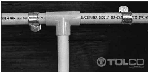
Tolco Single Fastener can function as a hanger, or as a restraining device by inverting the hanger and installing with the fastener mounting tab downward. Installing this type as a restrainer will prevent the upward movement of the sprinkler head during activation.
