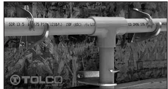
Tolco Stand-Off Hanger/Restrainer can function as a hanger or as a restrainer for installations where a standard offset is required. The Stand-Off Hanger can perform as both a hanger and restrainer on horizontal piping, and as a stabilizer for vertical sprinkler head drops. The manufacturer furnishes listed fasteners for use into wood.
