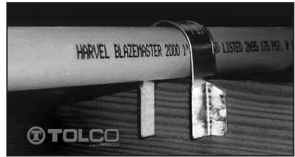
Tolco Hanger/Restrainer can function as a hanger or as a restrainer and can be mounted from the top or bottom of a beam. The fastener mounting edges are designed to allow the screws to be installed horizontally. This is a benefit when overhead clearance is limited.
